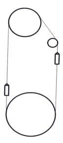
Determine for a nominal winding cycle the available stopping distance – as required by Directive C2 – from the stopping point, where the emergency brake would come on if the speed controller fails at the end of the full speed zone. Ensure that the emergency deceleration would not cause slip at the driving sheave wheel. Assume a friction force of 10 kN for each conveyance.
